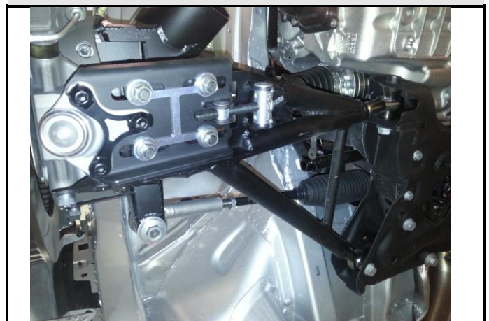
VII-E2) wishbone in its position
