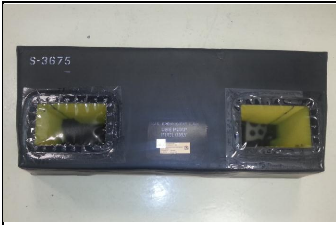
D1-1) Fuel tank dismounted
