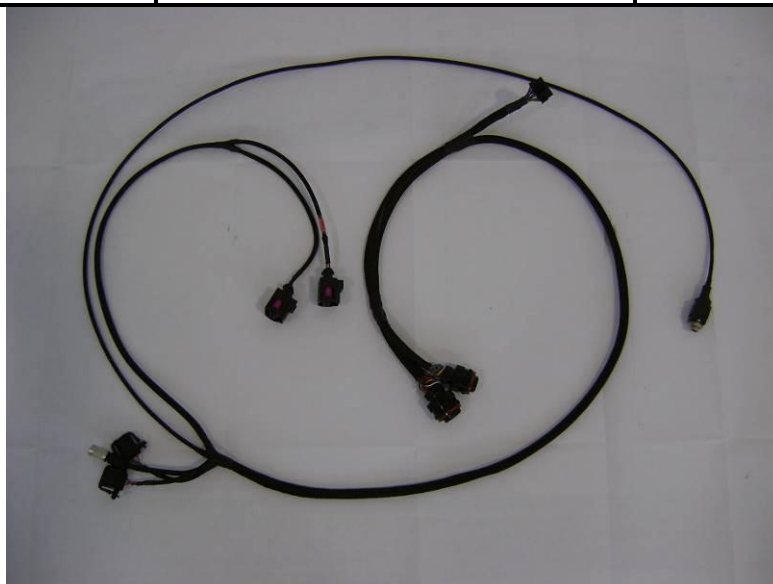
DASHBOARD AND LOGGER WIRE LOOM DISMOUNTED
