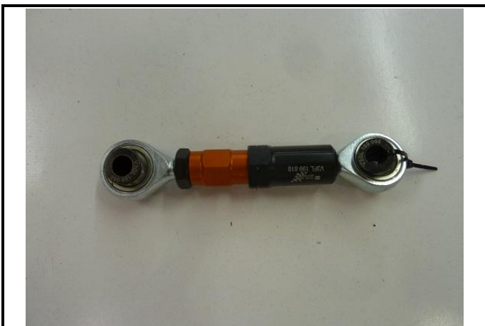
C2-3) Engine support 3 dismounted (photo)
