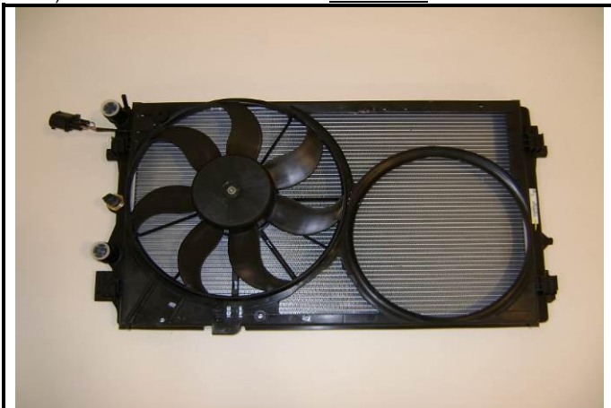
C13-7) Water radiator + fan carcass – dismounted
