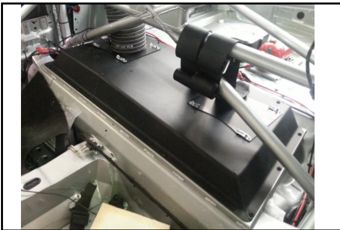
D1-3) Fuel tank in its location – with cover
