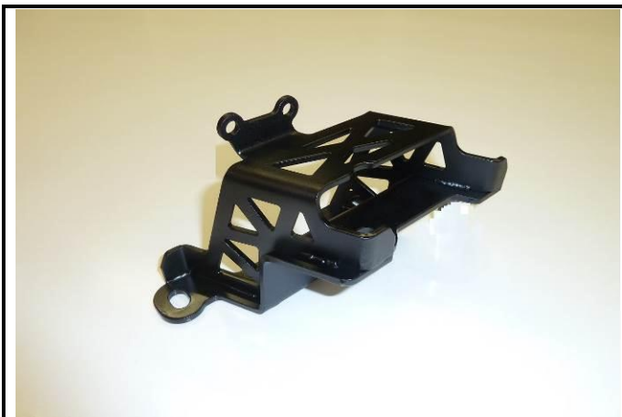
C2-2) Engine support 2 dismounted (photo)
