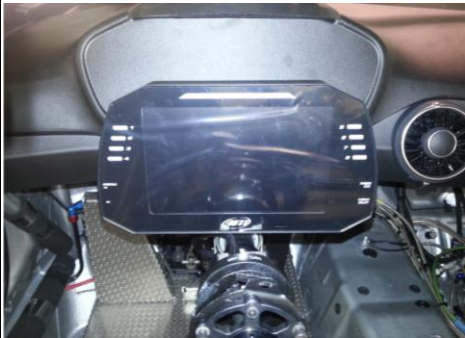
DATA LOGGING UNIT IN ITS LOCATION
