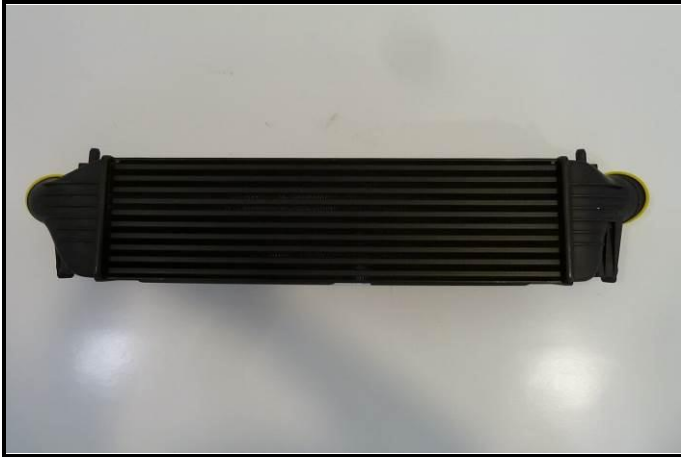
C15-8) Intercooler – dismounted
