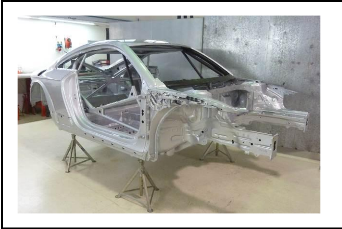
N1-3) Bare bodyshell – Cockpit seen from the right door
