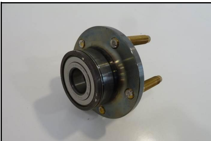
G4-1) Bare Wheel Hub – dismounted
