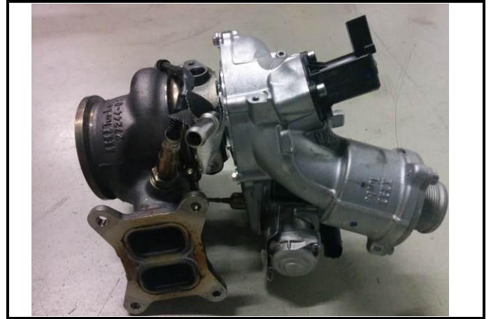
C15-2) Front view of complete turbocharger unit
