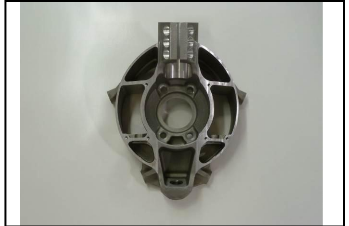
G3-2) Bare hub-carrier dimounted – dismounted
