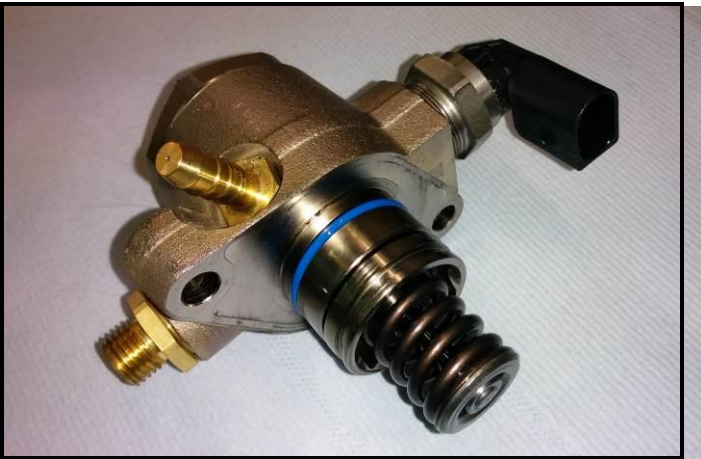
D2-1) Fuel pump(s) - dismounted
