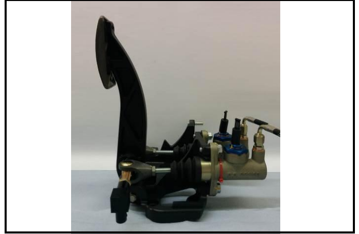
L2-2) Pedal box - dismounted seen from side
