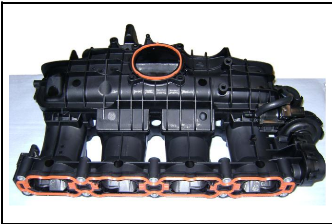
C11-1) Intake manifold - dismounted
