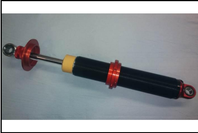
H6-1) Rear Damper – dismounted
