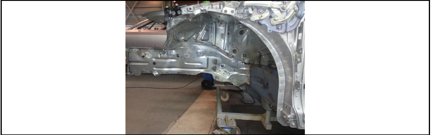
M8-6) Front wheelarch – modification of wheel arch
