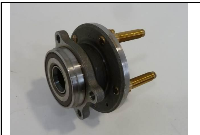
G4-1) Bare Wheel Hub – dismounted
