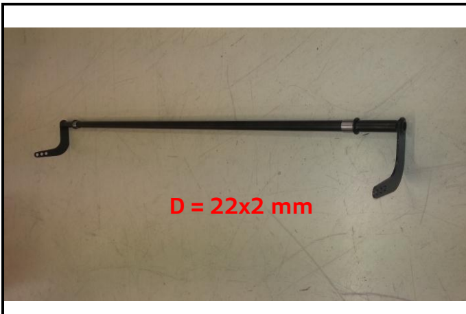
G6-3) Anti roll bar – dismounted
