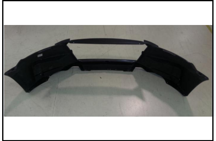
M9-2) Front bumper - dismounted inner side
