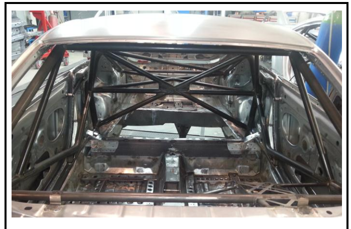
N1-4) Bare bodyshell – Cockpit seen from windscreen opening
